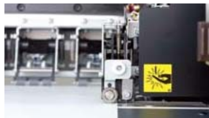
Head gap can be set step-less in 4 positions between 1.5 mm to 7 mm.
